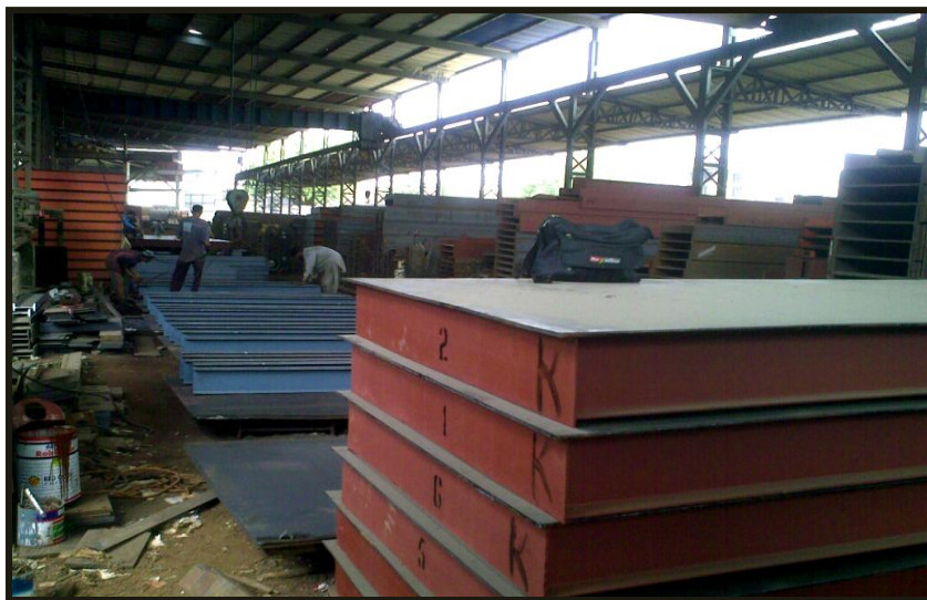
Figure 5: Fabrication of Weigh Bridge
